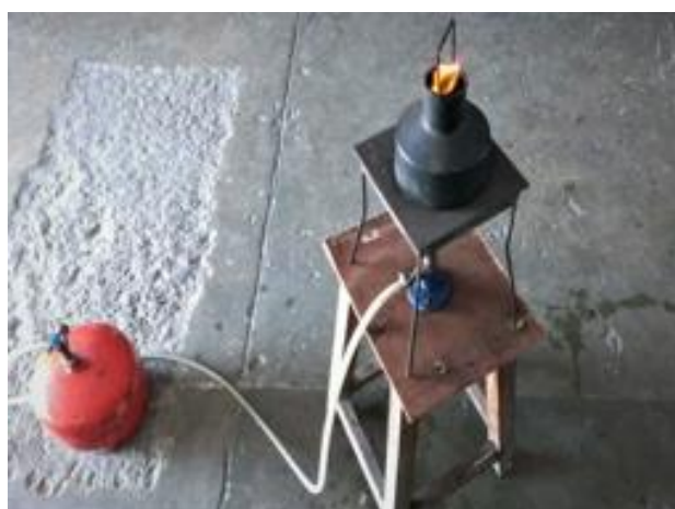
Fig. 14. Conradson Carbon Residue Apparatus.
