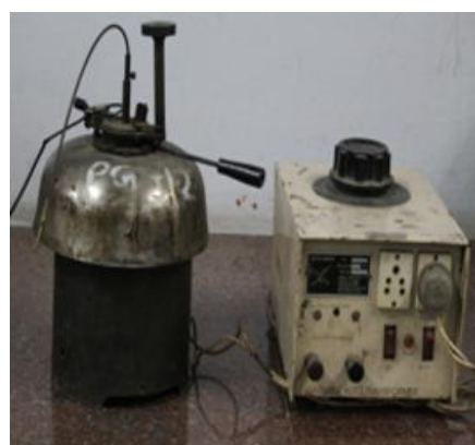
Fig. 6. Pensky–Marten's apparatus for flash point measurement.
