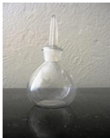
Fig. 2. Pycnometer for density measurement.
