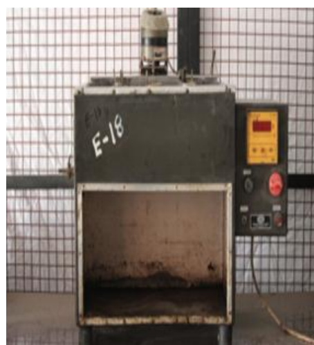
Fig. 4. Redwood viscometer for the viscosity measurement.
