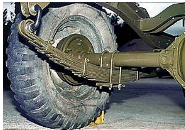
Fig. 1. Leaf spring (semi elliptical).
